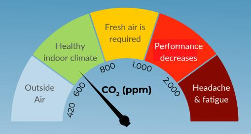
CO<sub>2</sub> measuring devices show when and for how long fresh air should be provided
